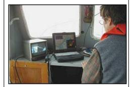
Survey operations showing use of RoxAnn<sup>TM</sup> and real-time video of the seafloor.
