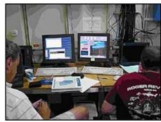
Operator station for the shallow and deep-water multibeam sonar systems. All system operation occurs through computer interface.
